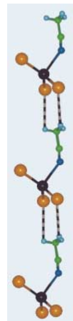
Figure 12. The chain of [\text{CuX}_3\text{NCCH}_3]^- ions in 3 . The \text{H-X} distances of the \text{C-H}\cdots\text{X} interactions (black and white stripes) are 3.37 and 3.45 \text{ \AA} .
